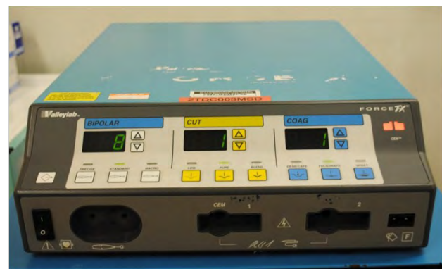
Figure 16: A diathermy generator.
